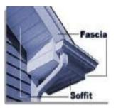
A finish member around the face of eaves and roof projections. Horizontal boards attached to rafter/truss ends at the eaves and along gables. Roof drain gutters are attached to the fascia.
